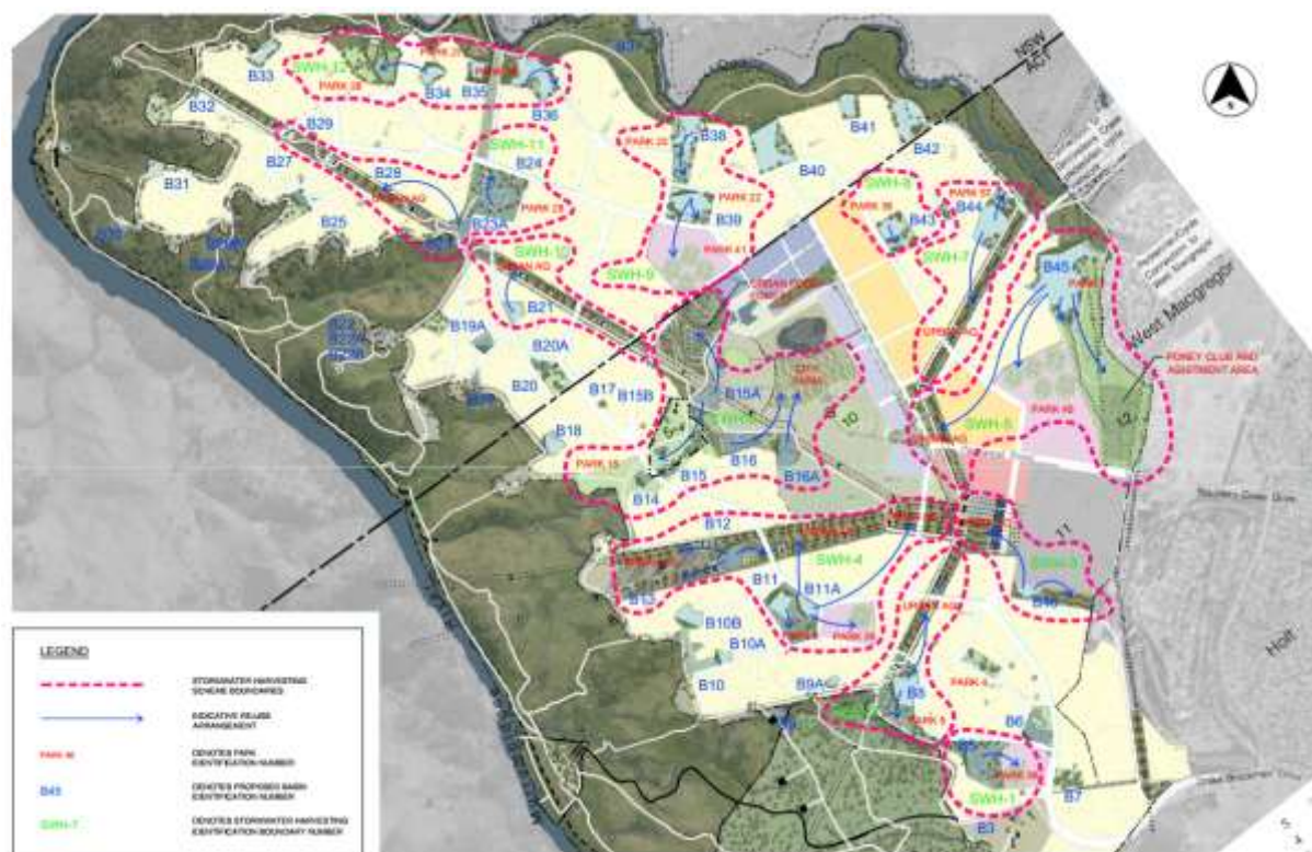
Figure 41 Decentralised local stormwater harvesting schemes option
